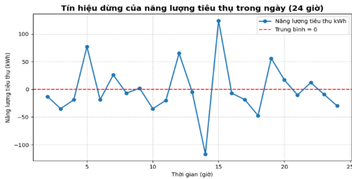
Figure 6. Stationary signal of daily (24-hour) energy consumption
